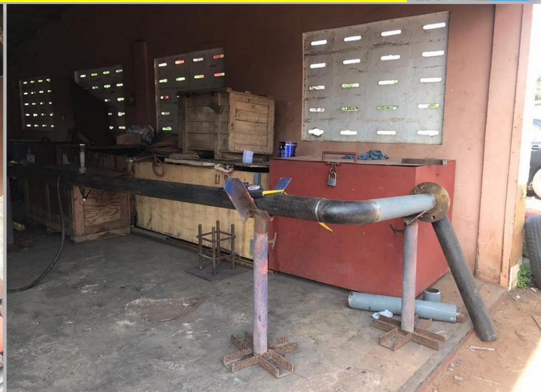
Fabrication of receiver, launcher, kicker, and bypass line for the pipeline inspection at CENPOWER from our Workshop
