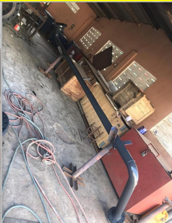
Fabrication of receiver, launcher, kicker, and bypass line for the pipeline inspection at CENPOWER from our Workshop
