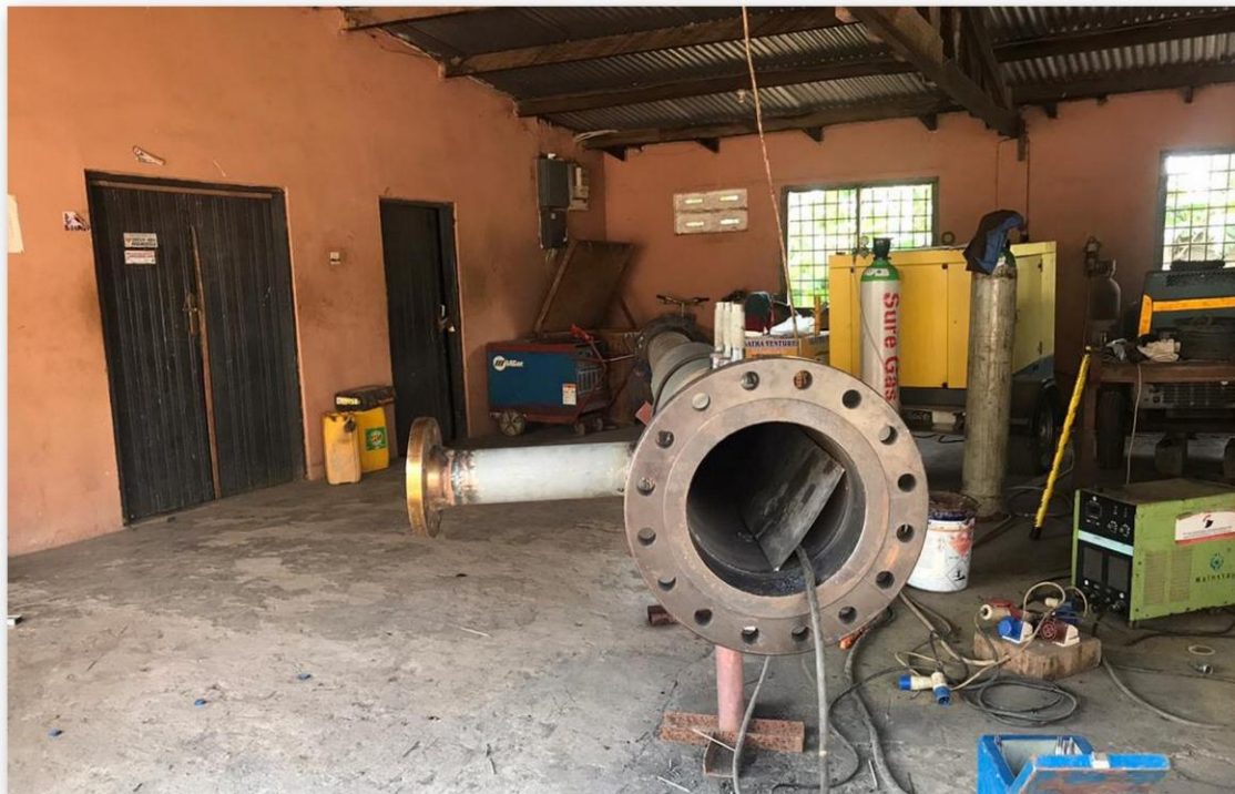
Fabrication of receiver, launcher, kicker, and bypass line for the pipeline inspection at CENPOWER from our Workshop
