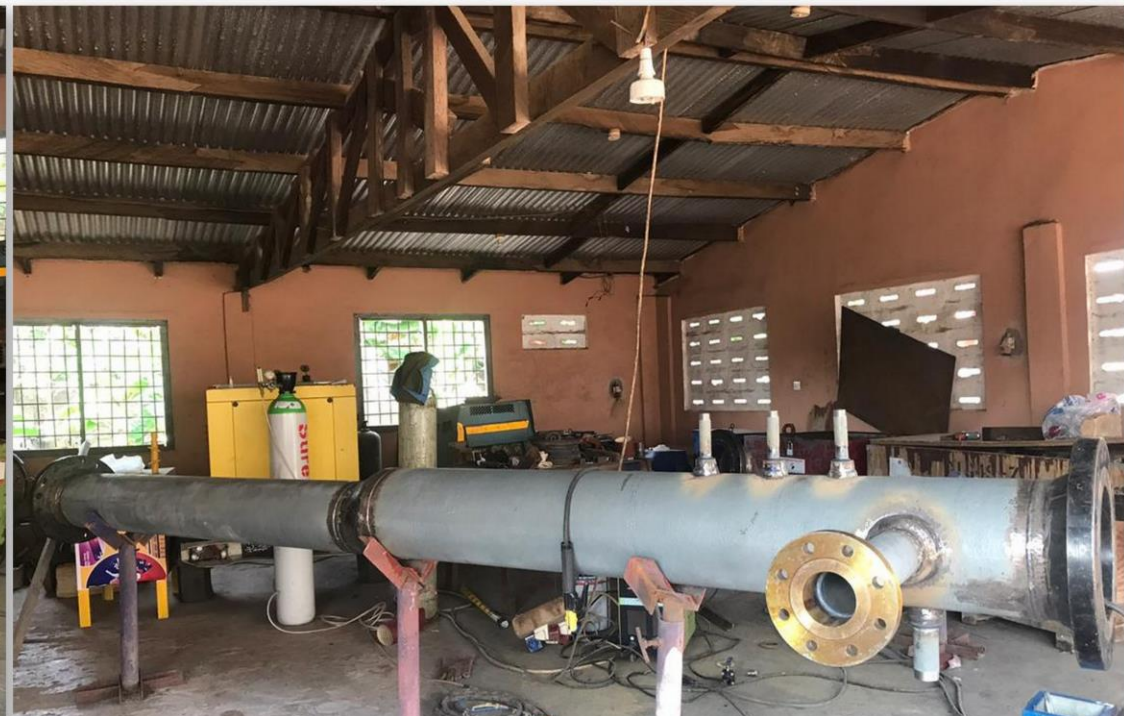
Fabrication of receiver, launcher, kicker, and bypass line for the pipeline inspection at CENPOWER from our Workshop
